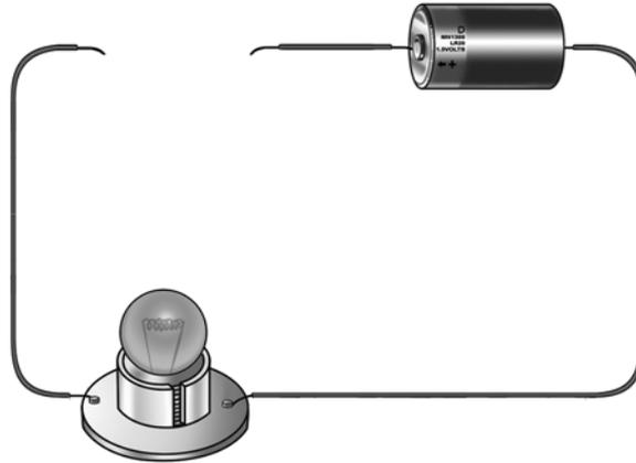
Tick the objects that would make the bulb light up if they were placed across the gap in the circuit?
